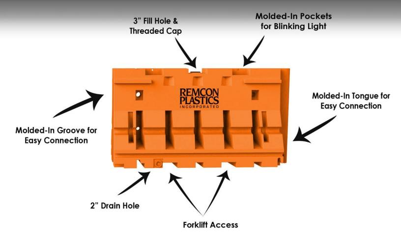
Remcon's GUARDSAFE 42 barrier is a water-filled Longitudinal Channelizing Device (LCD) ideal for traffic and pedestrian channelization in almost any environment. The barricade is manufactured with rotationally-molded polyethylene, which allows it to withstand the harshest weather conditions and resist dents and cracks.
