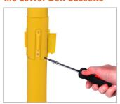
Step 1: Remove post retaining screws
