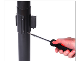
Step 1: Remove post retaining screws
